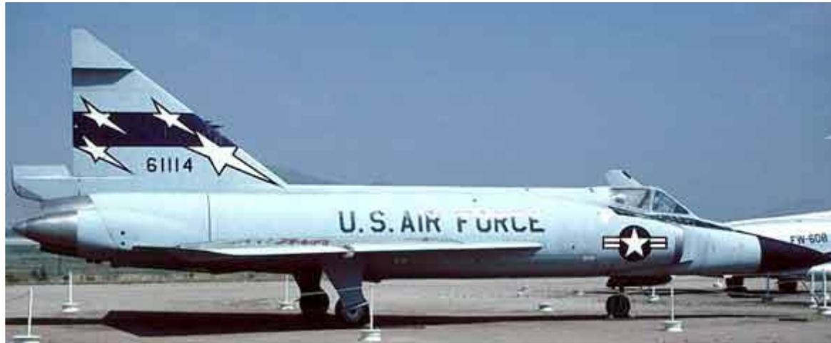
The **F-102** was the world's first supersonic all-weather jet interceptor and the USAF's first operational delta-wing aircraft. Its primary mission was to intercept and destroy enemy aircraft. In a wartime situation, its electronic equipment would locate an enemy aircraft, then radar would guide the plane into position attack. Then, electronic fire control system would automatically fire the **F-102**'s air-to-air rockets and missiles.
