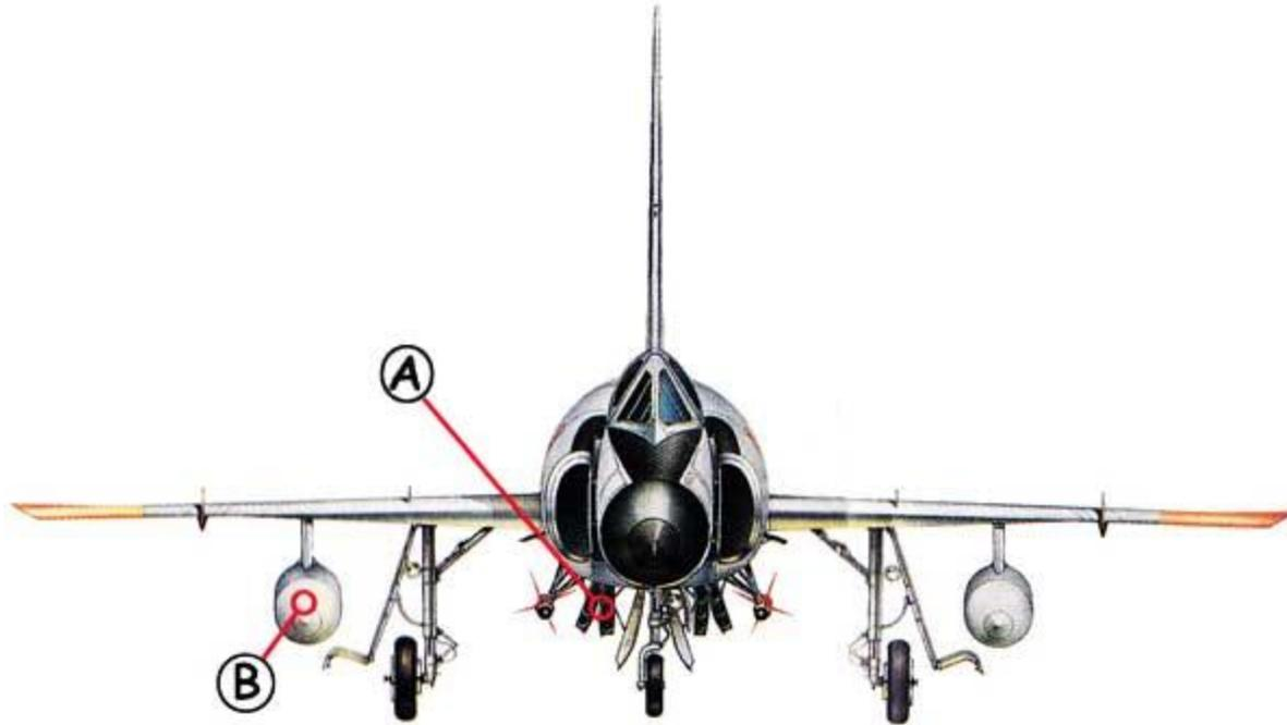
A: In addition to the Falcon missiles, the F-102 carried 25 unguided rockets.
