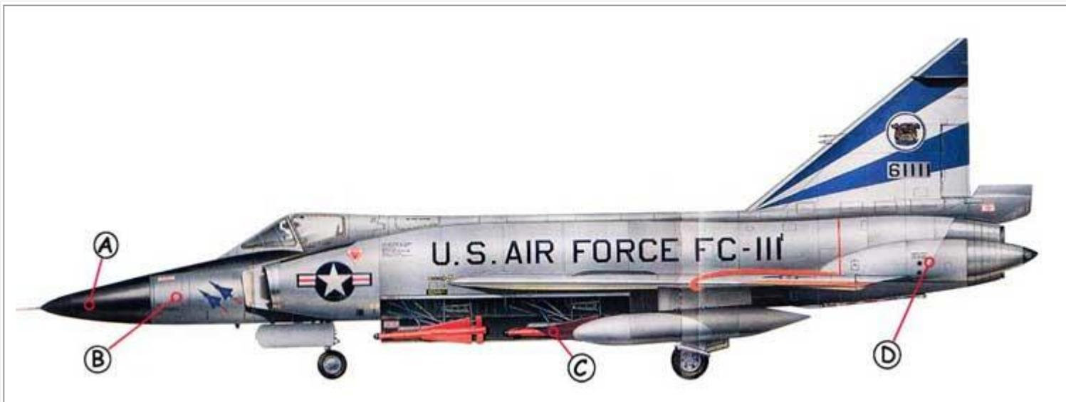
A: The radar component of the Hughes MG-10 fire-control system could track several airborne targets simultaneously at ranges of up to 30 miles, and lock on individual aircraft around 15 miles.
